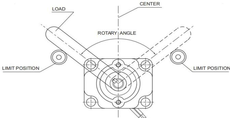
Installation diagram of limit device
