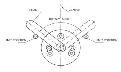
Installation diagram of limit device
