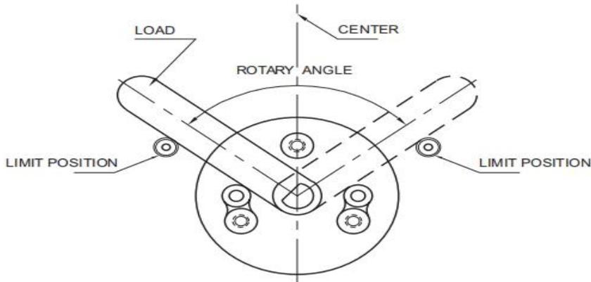
Installation diagram of limit device
